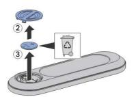
Insert a new CR2032 battery. The device beeps (1x) and the blue LED on the lateral control panel lights up for 4 seconds.
