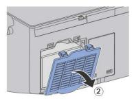
4 Remove the used filter from the opening. Then insert the new filter.
