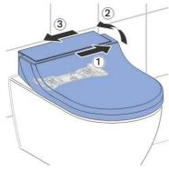
Turn the device a little in a clockwise direction until you have access to the filter cover.
