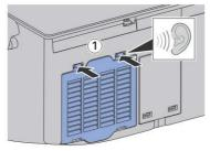
6 Mount the device on the base plate. Ensure that it is safely engaged.
